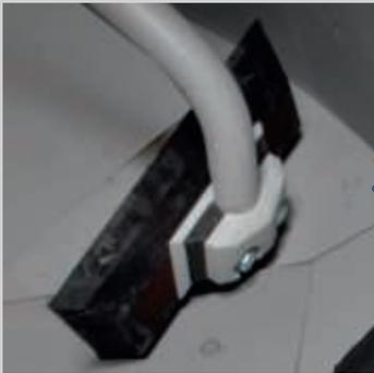
The mixing shovels can be turned, so that the lifetime is extended. Mixing arms have a diameter of 52 mm, which gives a long service life.
