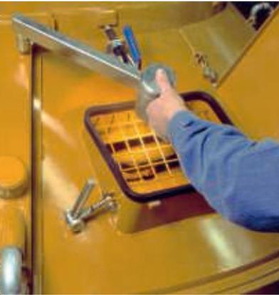
Lamp for inspecting the mixing cycle.
