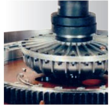
Mixers from 1125 litre have a hydraulic coupling so that they can be started under full load.
