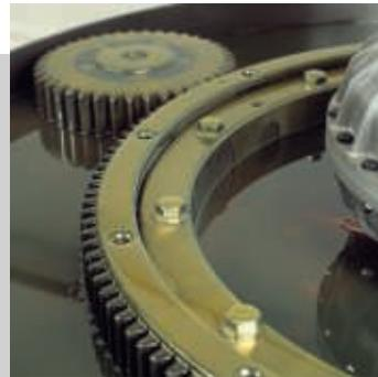
The Haarup gearbox with its open oil sump absorbs any transmitted heat which means no temperature measurement is necessary.
