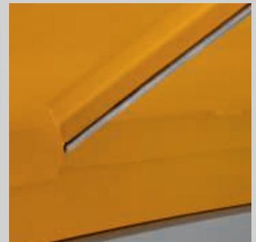
The plate covering of the mixing pan is designed with labyrinth seals ensuring optimum density and at the same time fast cleaning.
