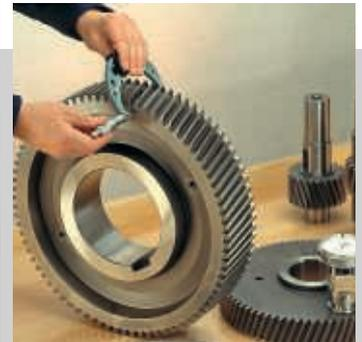
The gearbox is fitted with a special ring gear, hardened and ground toothed gears installed in spherical or conical roller bearings.
