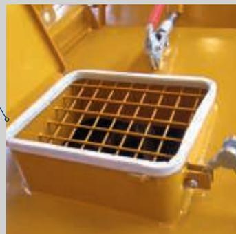
A concrete inspection door with safety grill in a mixer lid.
