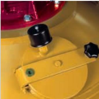
The inspection door makes it easy to inspect the gearbox and the oil level.
