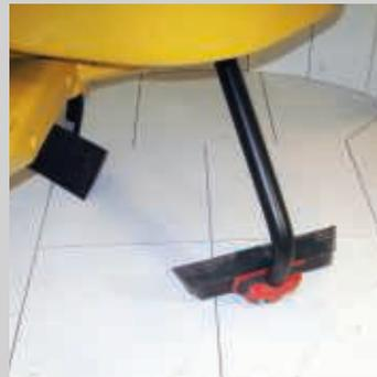
Specially hardened fixing bolts for wear plates, which are completely flush to the pan, ensure that the mixing shovels and wear plates have a long lifetime.
