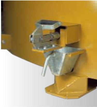
Equipment for concrete samples.
