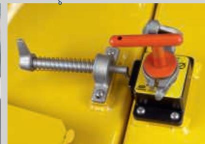
Mixer lids are fitted with relevant safety switch systems. When incorporated in the control system they will prevent the mixer running when the lids are opened.
